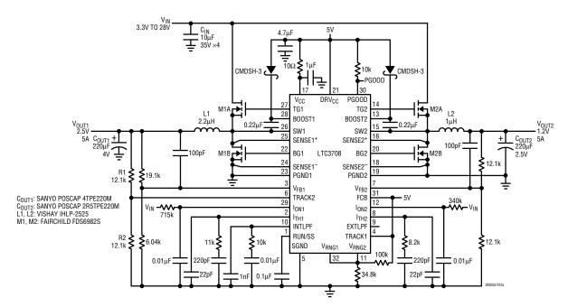
Figure 1a. Dual Power Supply with  $V_{OUT2}$  Tracking  $V_{OUT1}$
