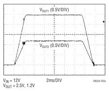
Figure 2b. Ratiometric Tracking (R1 = 19.1k, R2 = 6.04k)
