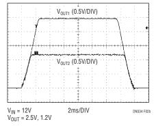
Figure 2a. Coincident Tracking (R1 = R2 = 12.1k)
